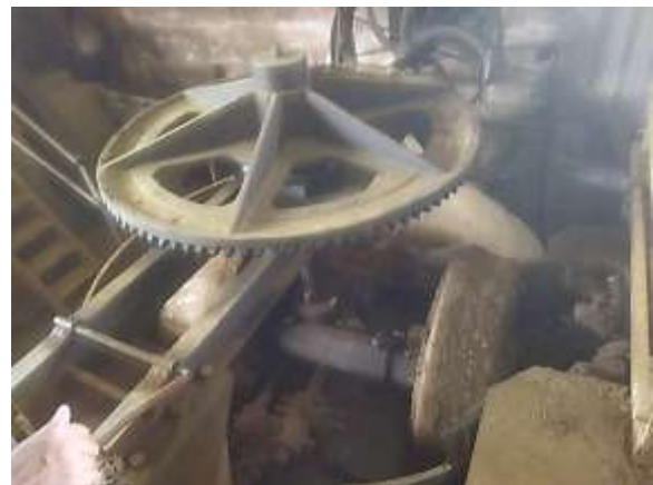
Figure 4. The speeder used for mixing the clay at the beginning of the manufacturing process.
