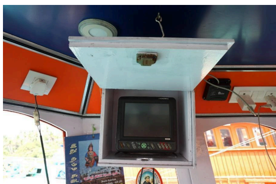
Figure 8. Echo sounder mounted on the wheel house ceiling. Image: JANAL Archives 2023.
