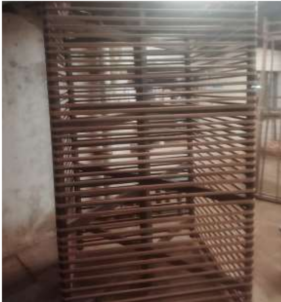
Figure 5. The tool on which the process of warping, the second process in the three-step making of the Kasargod Saree, takes place, known in Malayalam as the ' paav maram .' Image:
