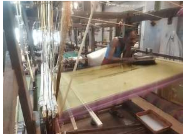
Figure 6. A worker engaged in the process of 'sizing the warp', that is, applying the adhesive agent while the still loom. Image:
