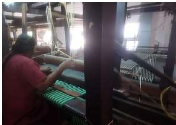
Figure 9. A worker using the loom to make a tuvarth (bath towel). Image:
