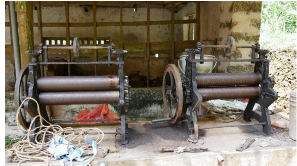
Figure 2. Rollers used to squeeze the rubber sheets. Image: JANAL Archives 2023
