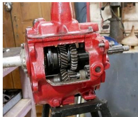
Figure 5. The inside of a gearbox cut out to show the working at the Four Wheeler Service Technician (FST) laboratory, Rahmaniya VHSS. Image: JANAL Archives, 2023.
